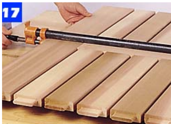
Glue and clamp a side rail to the center rail. One clamp, carefully centered, should provide enough force.
