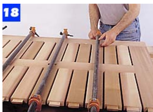
Glue and clamp a side rail to the center rail. One clamp, carefully centered, should provide enough force.
