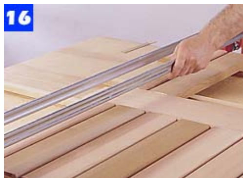
A second set of slats is glued and clamped to the center rail. Again, use one clamp in the center of each slat.
