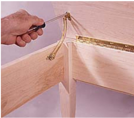
10--Sequence is important when attaching the top's support hardware. Attach it to the apron first, then the top.
