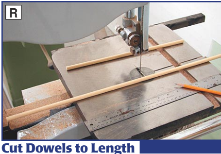
Cut Dowels to Length
