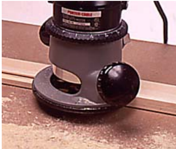
14 --Use a router with a piloted slotting bit to cut the slots in the upper door frames for the plastic glass-retaining strips.
