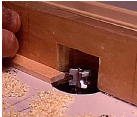
14 --Use a router with a piloted slotting bit to cut the slots in the upper door frames for the plastic glass-retaining strips.
