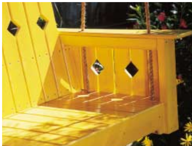
A continuous length of sturdy rope runs through armrests and frame. Note short, notched back board under armrest.
