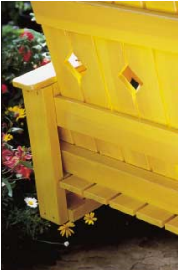
Back brace secures in top rear corner of side frame. A slice cut from its front face helps create the comfortable angle of the back.
