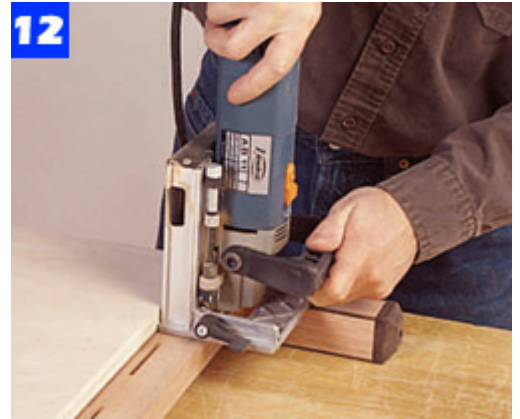
Lay out the plate slots in the table sides for attaching the bottom shelf. Use a straight board as a guide for the joiner.
