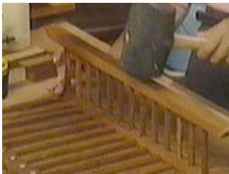
Use a rubber mallet to help seat the dowels
