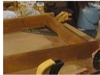
Glue and nail the sides to the bottom shelf
