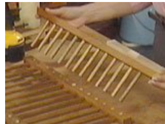
Start from one end, inserting the shelf dowels into the holes
