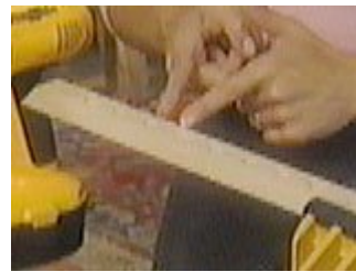
Space the holes one and one-quarter inches apart, measured centre to centre
