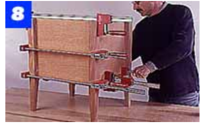
Use bar clamps at the location of each joining plate to evenly distribute pressure when assembling the table case.
