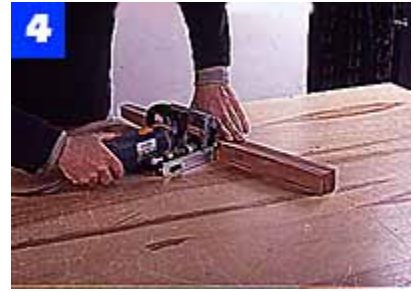
Mark joining-plate centers on each leg, then cut the plate slots. Hold the leg firmly to the work surface while doing this.
