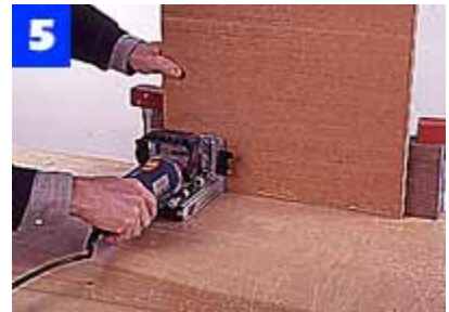
Clamp a tall backstop to the workbench, and hold a panel firmly against it. Cut joining-plate slots in the panel edge.
