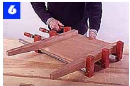
Assemble two legs and one table side with glue and joining plates. Apply pressure with a clamp at each plate location.
