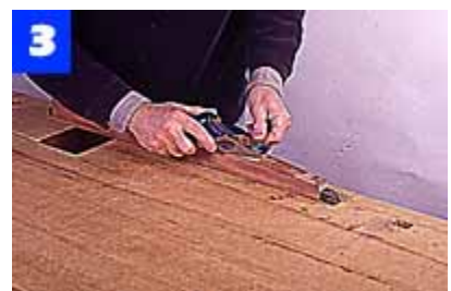
Clamp each leg to the workbench top. Next, use a block plane to remove saw marks and refine the leg taper.
