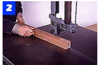
Mark the taper on two faces of each leg, then cut the tapers on a band saw. Stay on the waste side of the pencil line.
