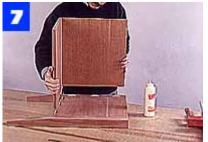
Glue and clamp together the table back and bottom. Take this subassembly and join it to the leg-side subassemblies.
