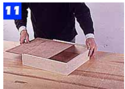
Cut the plywood drawer bottom to size. Once the glue has cured, slide the drawer bottom into its groove.
