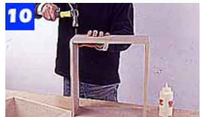
The drawer box is built with rabbeted and grooved pieces. Assemble the box with glue and finishing nails.
