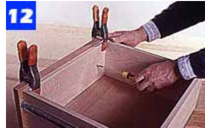
Clamp the drawer front to the drawer box, bore pilot holes, and attach the front with flathead screws.
