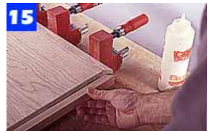
Glue solid edging to the desktop panel. Let the edging overhang the panel faces, and plane it flush after the glue sets.
