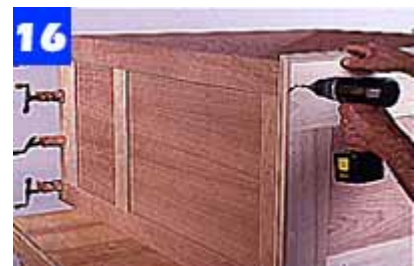
After using glue and plates to join the top to the side frames, position the desktop at the bottom of the sides and screw it in place.
