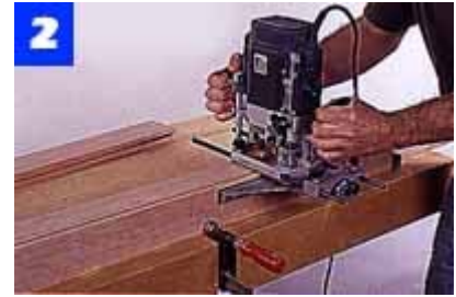
Use a router and edge guide to cut mortises and panel grooves. Clamp together stock to provide a firm base for the router.
