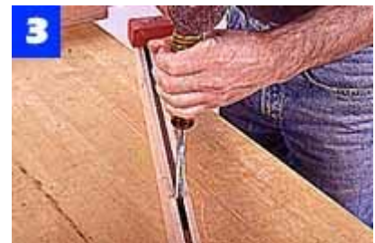
After the grooves are cut, use a sharp 3/8-in.-wide chisel to square the ends of each mortise in the side and door stiles.
