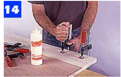
Build up the bottom edges of the desktop by gluing 1/4-in.-thick spacers to the panel. Keep the strips flush with the panel edges.
