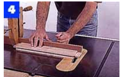
Use a dado blade in the table saw to cut the tenons slightly oversize. Then, pare them to the exact size with a sharp chisel.
