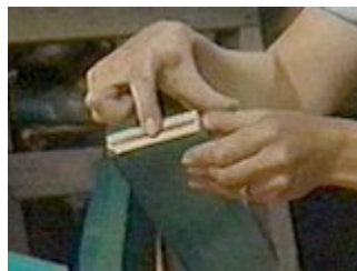
Slot made for the biscuit in the end of an apron piece
