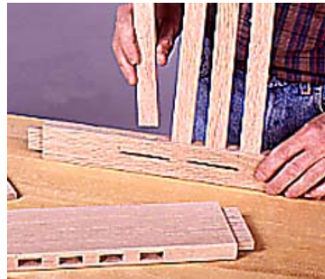
7--Test fit the side slats in the rail mortises. Sand or trim the joints, if necessary, to achieve a tight fit for each slat.
