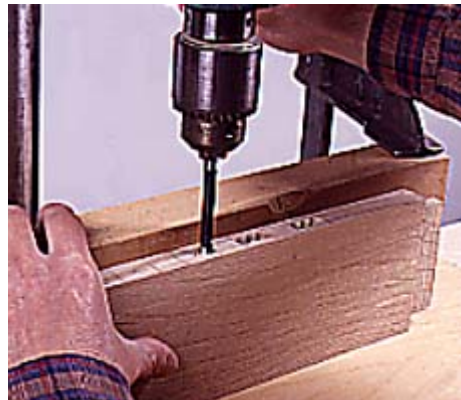
4--Cut the slat mortises in the rails using a drill press to remove most of the waste and a sharp chisel to finish the cuts.
