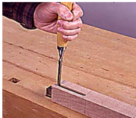
2--When the routing is done, carefully square the ends and flatten the sides of each mortise with a sharp chisel.
