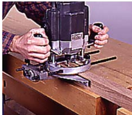
1--Use a router with an up-cut spiral bit and an edge guide to cut the rail mortises in the table legs. Make several passes.
