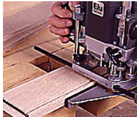
15--Cut a dado between the dovetail slots on the drawer face for the bottom panel. Cut matching dados in the drawer sides.
