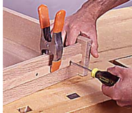
17--Slide the drawer bottom in place and attach it to the back with screws. Also, screw the guide strips to the sides.
