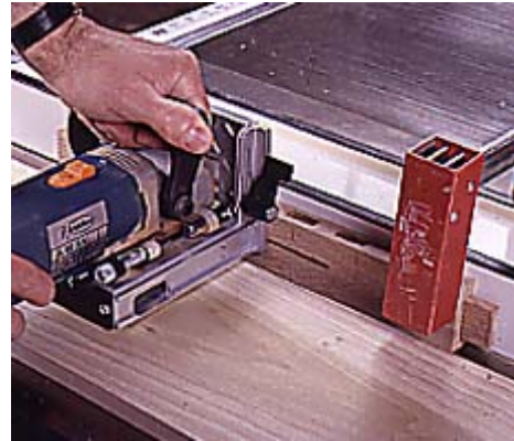
6--Clamp the bottom rails to your table saw fence. Then use a plate joiner to cut joining slots in one side of both rails.
