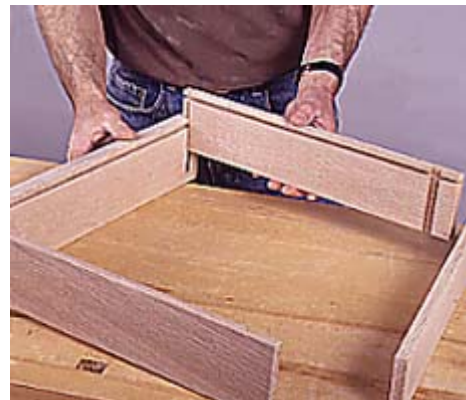
16--Apply glue to all the drawer joints, then clamp the box together. Reinforce the side-to-back joints with brads.
