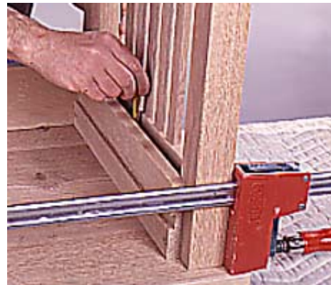
18--Center the base over the top and mark the fastener holes. Then bore pilot holes in the top and attach the base.
