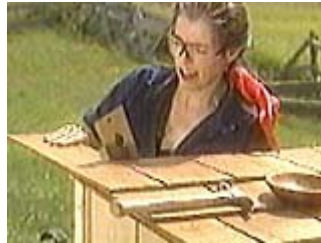
Use a hand saw to cut off the excess at the back
