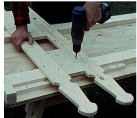
4--Build an assembly table with stops to position rails. Use spacers to locate pickets and attach with two screws per rail.
