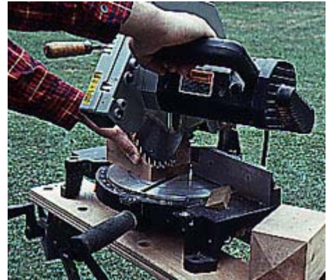
6--Use a power miter box to cut top blocks to size and shape. Set the saw for 23 degrees and trim to centerlines marked on the block end.
