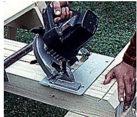
1--Gang together picket blanks and use a circular saw set at 45 degrees to make most of the cuts for the rough picket shape.
