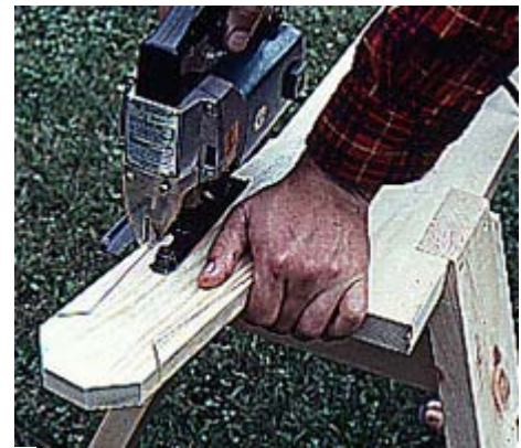
2--Finish the rough picket outline by making the longer side cuts on individual pickets with a sabre saw.
