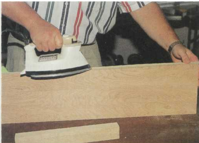
15 Veneer tape is simply ironed on to the visible edges of the MDF board.
