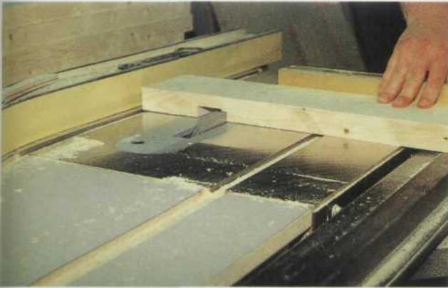
6 Remove the waste from the dovetail pockets using the dado set-up.
