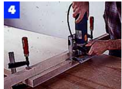
Cut joining-plate slots in case parts. Clamp a guide across the panels to help position the joiner for slots in the panel faces.
