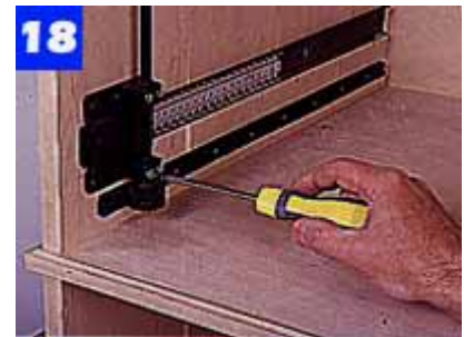
Screw the pinion-wheel/mounting-block assembly to the door slide. Detailed instructions are included with the hardware.
