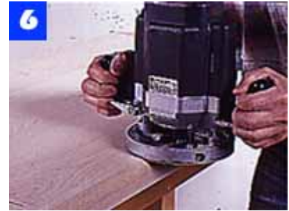
Use a 5/8-in.-rad. rounding-over bit to shape the bottom edge of the case top. Rout a 30-degree chamfer around the edge.
