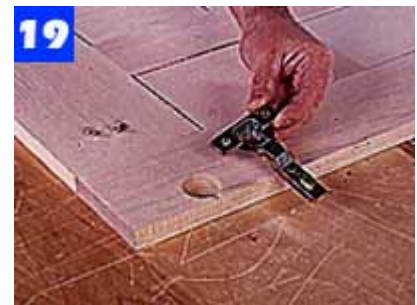
Bore 35mm-dia. recesses in the door stiles for the hinge cups. Then, install the hinges to the doors and adjust for proper operation.
