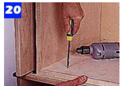
After assembling the case insert, bore pilot holes and fasten it to the cabinet top and middle shelf with screws.
