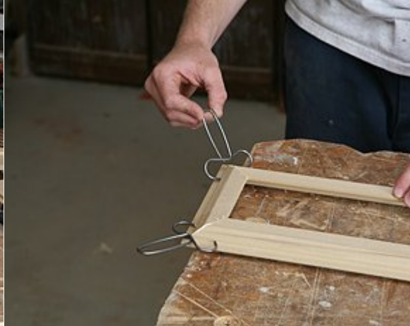
Swivel the spring clamps up out of the way.
