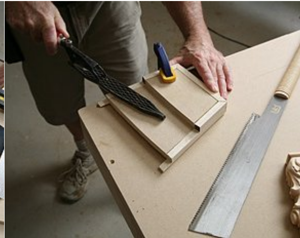
Using a pull saw and Shinto rasp, I notched the molding for each layer of 1/2 in. mdf.
