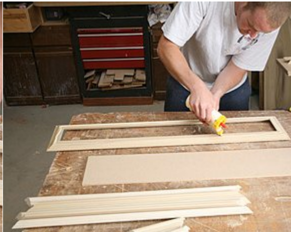
Apply glue to the back of the molding.
