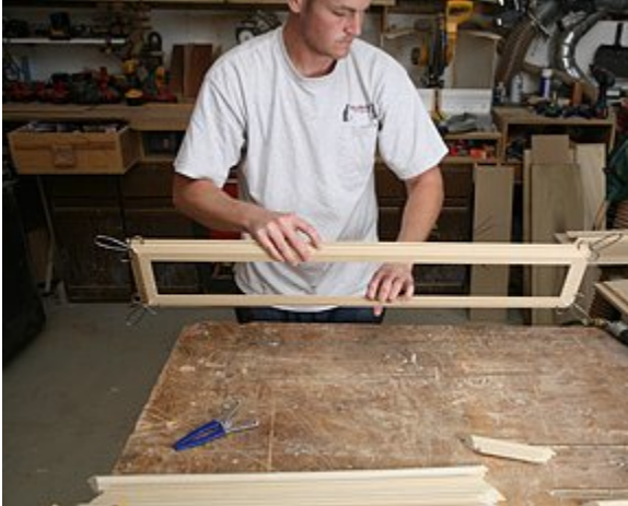
Once the spring clamps are positioned on each corner, flip the molding over.
