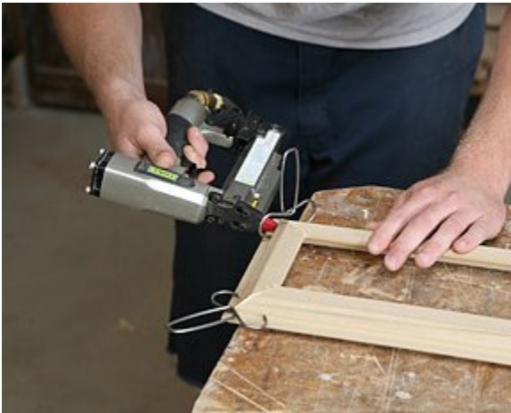
And nail off the miters with two brads in each corner.
