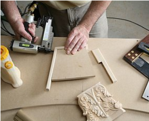
I surrounded the backboard with 1/2 in. molding.
