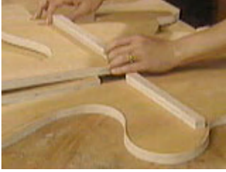
Attach three quarter inch strips on the sides to support the seat
