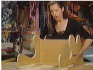
Pull all the pieces into position, clamp and screw the pieces together
