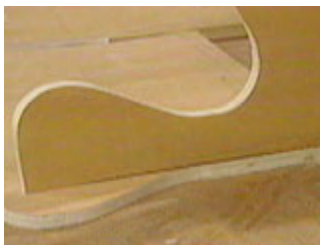
Notch the sides to accept the back
