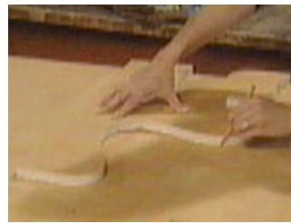
Trace the second piece onto the plywood
