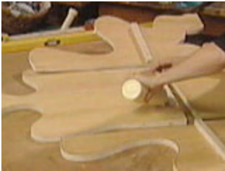
Lay out all parts for assembly and apply glue to surfaces that touch
