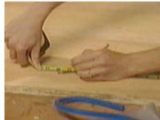
Mark the height for the seat sides
