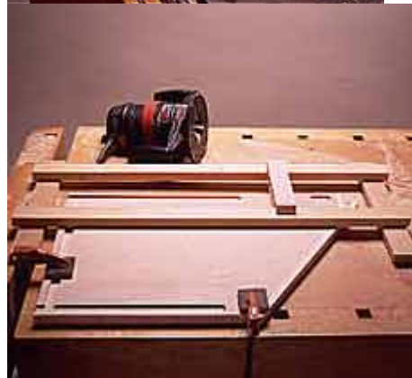
4--Cut grooves and dados in the end panels with a router. The block is tacked across the rails to stop the cut.
