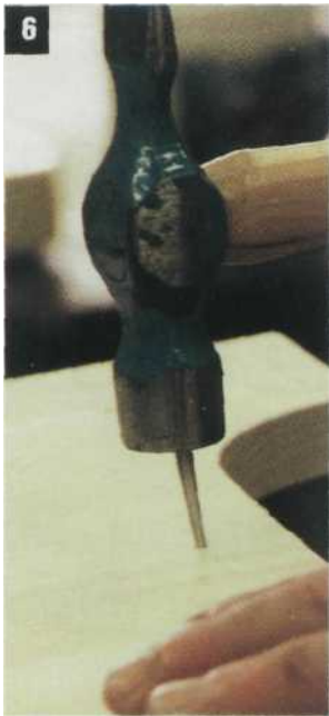
Driving a cut nail, showing the wide dimension of the nail, is oriented along the grain of the wood you're nailing through
