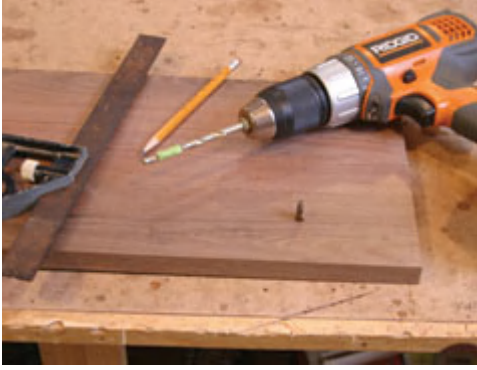
Shelf pin holes in the sides provide for shelves if the case is to be a trophy or bookcase.
