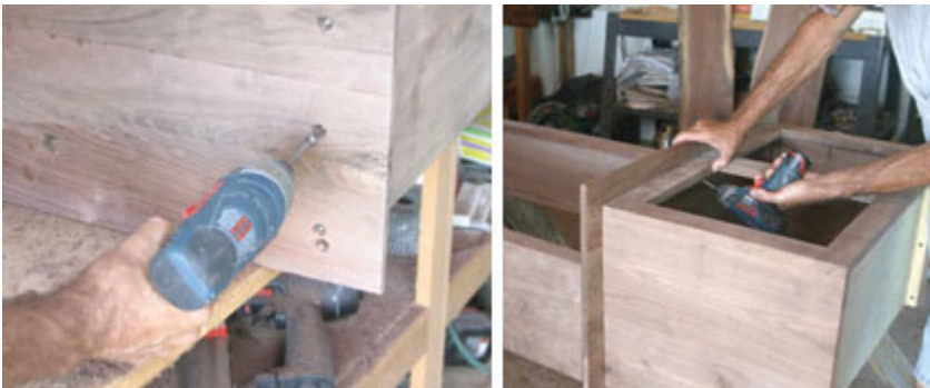
Left: The bottom section top is fastened to the top section with screws from the underside.
