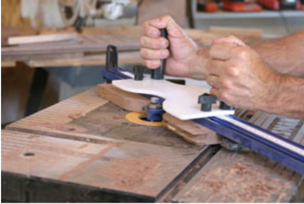
Bottom raised panel doors are created using Woodline's new Raised Panel Door System.
