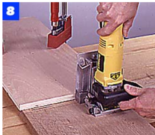
Cut plate slots in the case top and bottom for the partition. Clamp a guide board in place to align the plate joiner.
