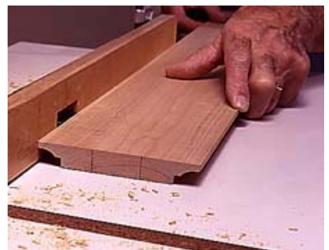
7--The dentil molding is cut using a router with a guide strip screwed to its base. The strip rides in the previously cut dado.
