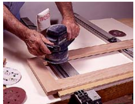
14--Sanding door rails and stiles can be tricky. Use a random-orbit oscillating sander to avoid crossgrain sanding.
