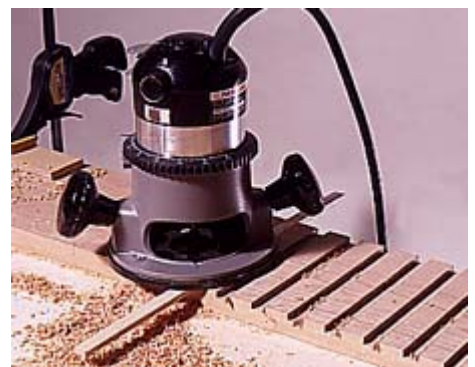
7--The dentil molding is cut using a router with a guide strip screwed to its base. The strip rides in the previously cut dado.
