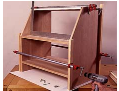
6--Glue and clamp the case sides to the horizontal panels and drive screws into the upper and lower panels.
