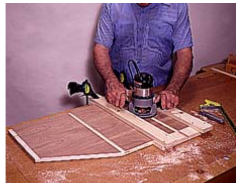
3--Use a router with a straight bit and a parallel fence jig to cut the rabbets and dados in the case sides.
