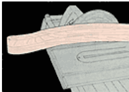
Fig. 1 Sand the two rockers to identical contours using the pad sanding technique.
