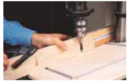
Another view of the drill-press table. Here I'm cutting pocket holes in a table apron.
