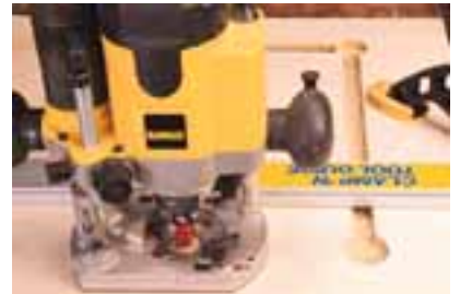
ROUT THE GROOVE The grooves for the T-slot track allow the fence to be used left-to-right and front-to-back on the table to take advantage of the built-in tilting feature of the existing table.
