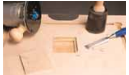
RABBET FOR THE INSERT After cutting the hole with a jigsaw, the opening is rabbeted using a bearing-piloted router bit. Then chisel the corners square and fit the replaceable center tightly into the rabbet. Make a couple extras.
