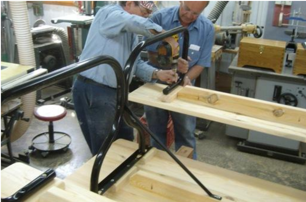
Step 4: Assemble the Picnic Table - Select the Metal Legs and Assembled Pieces from Step 3
