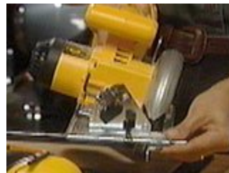
Use a ripping guide for straight cuts
