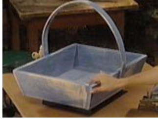
Finished trug with compound angles and bent-wood handle
