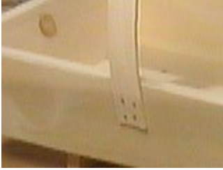
Use decorative copper nails to secure the handle
