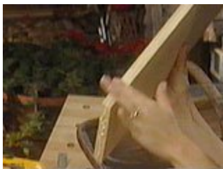
Bevel and then apply glue to the edges of the bottom boards
