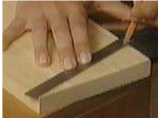
Using a protractor, scribe a 15 degree line
