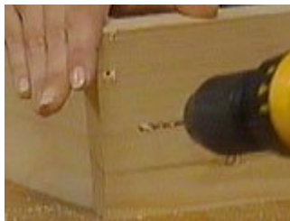
Pre-drill before nailing
