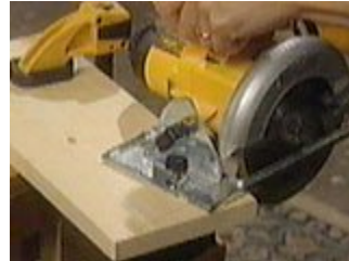
Cut along the line with a circular saw
