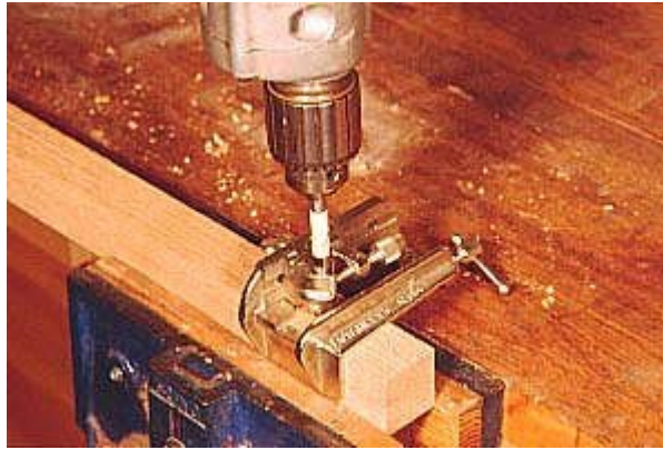
Photo 2 The dowel jig shown is the Stanley model, a versatile dowel jig. Another versatile dowel jig is the Dowl-It jig, which you can see by clicking here .
