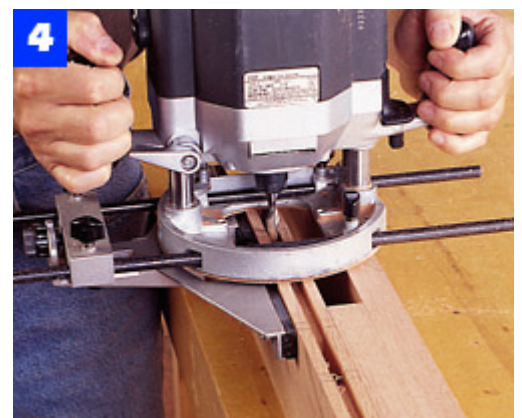
Readjust the bit depth and rout the panel grooves. Spare pieces clamped to the work help support the router.
