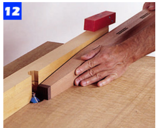
Use a router table to chamfer the leg corners. At the inside corner of each leg, chamfer only the tapered section.
