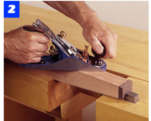
Use a sharp plane to smooth the tapers. Reverse the direction of the plane at the bottom to avoid splintering the foot.
