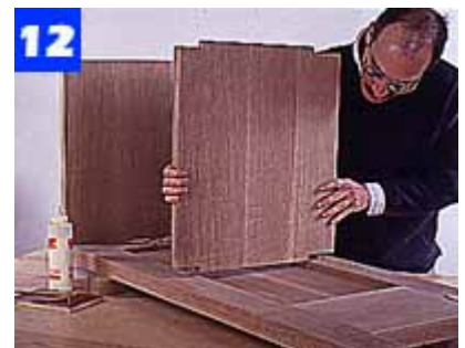
Apply glue to the slots, dowel holes, joining plates and dowels, then assemble the shelves to one case side.
