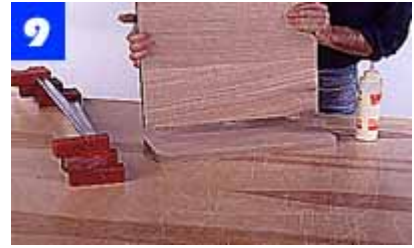
After you have cut the joining-plate slots in the top shelf and back rail, test fit the pieces, then glue and clamp them together.
