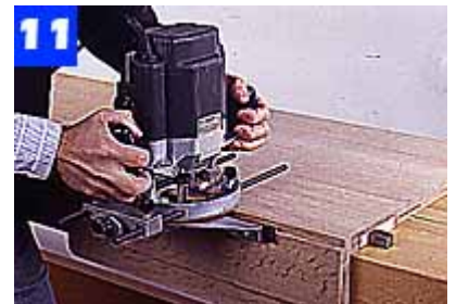
Using the router with an edge guide, make two or three passes, and cut the rabbet on the top rail/shelf assembly.
