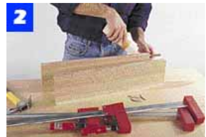
To ensure a properly bonded joint, apply glue to the joining-plate slots, the board edges and the joining plates.
