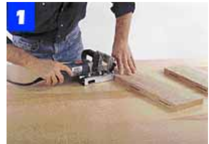
Cut joining-plate slots in the boards' edges. The plates keep the boards aligned while they are being glued and clamped.
