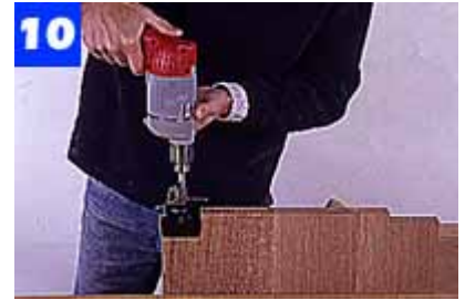
Make the center case shelf, cut the notches in its ends, and bore the holes in the notches using a doweling jig.
