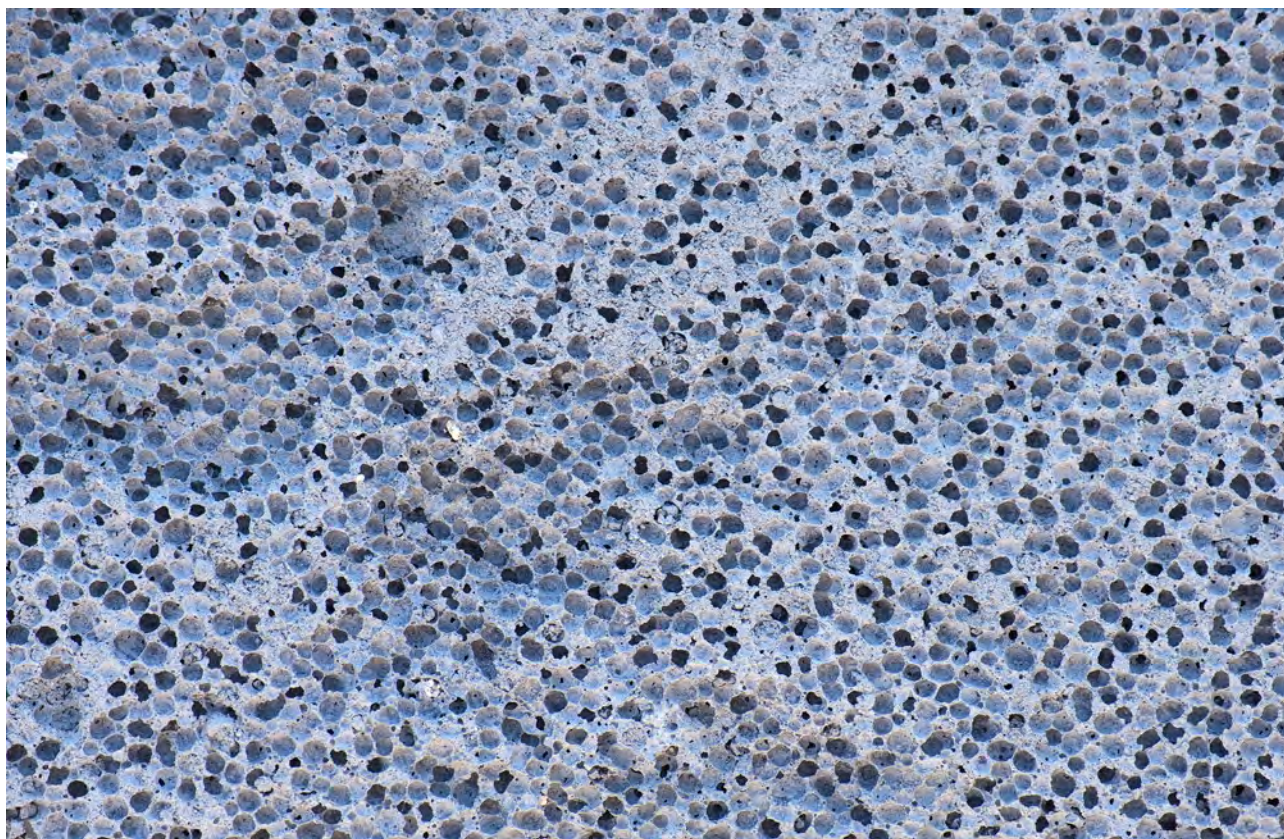
Lightweight foamed concrete is a substitute material for traditional concrete in building construction
