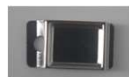
Figure 1: The stainless steel coupon used for the culturability assay. Bacteria was inoculated onto the centre of the coupon.
