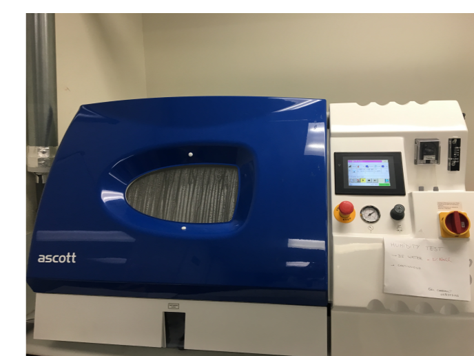
Figure 7. Salt spray chamber used to test corrosion resistance
