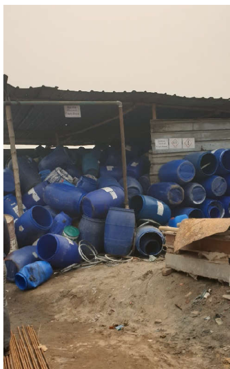
Figure 10.14 Sign saying "hazardous chemicals: empty drums", while they are disposed together, in an open place
