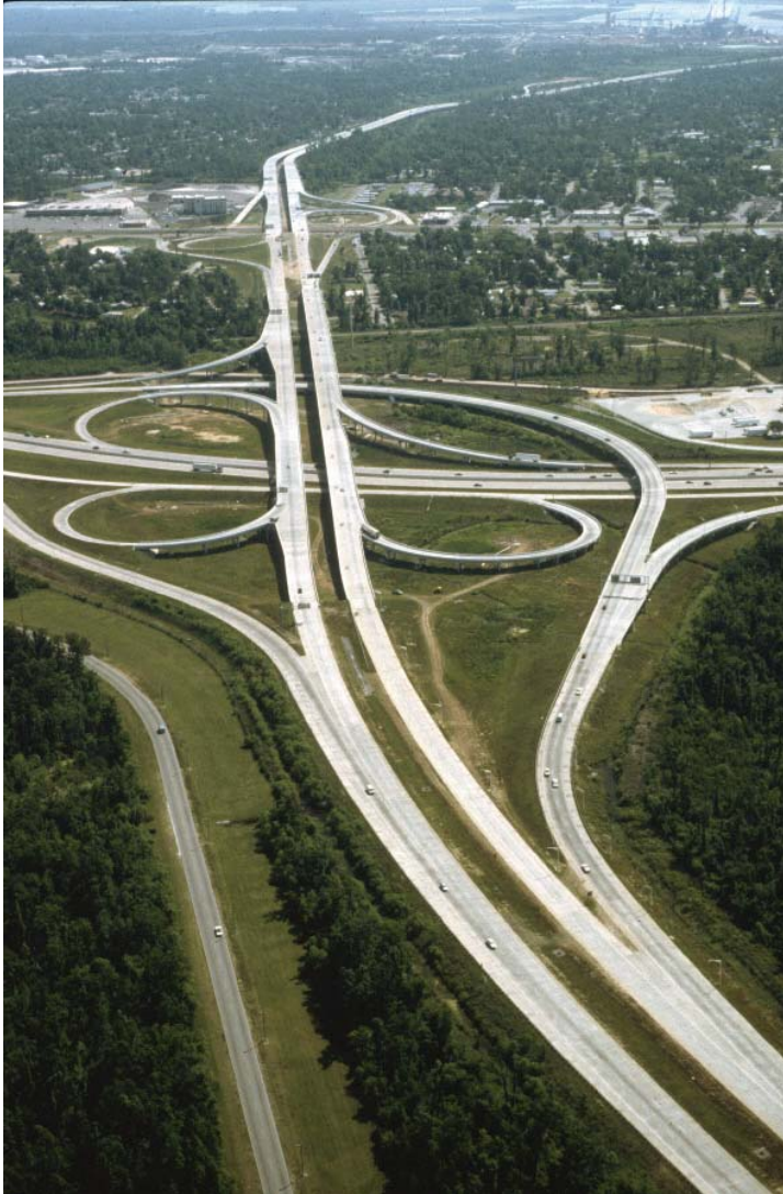
Figure 10-42. Cloverleaf Interchange with Semidirect Connection
