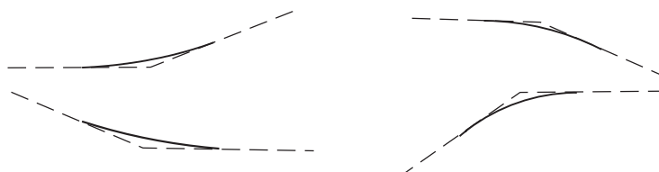
Figure 3-16. Diagrammatic Profiles Showing Methods of Attaining Superelevation for a Curve to the Right (Continued)
