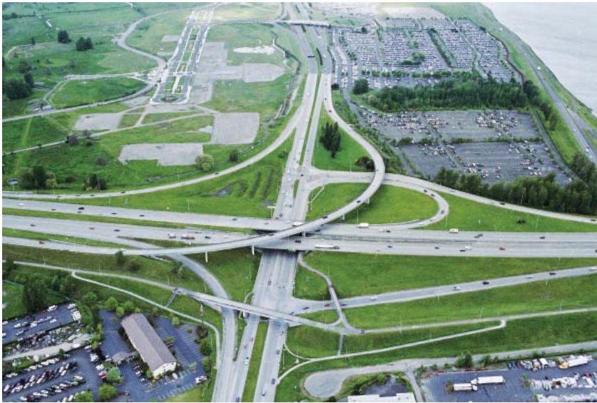
Figure 10-40. Four-Leg Interchange, Diamond with a Direct Connection
