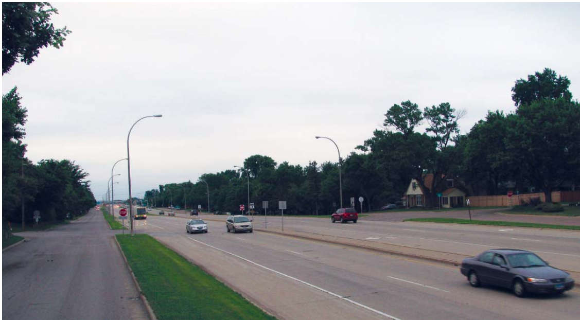
Figure 7-11. Divided Arterial Street with Two-Way Frontage Road
