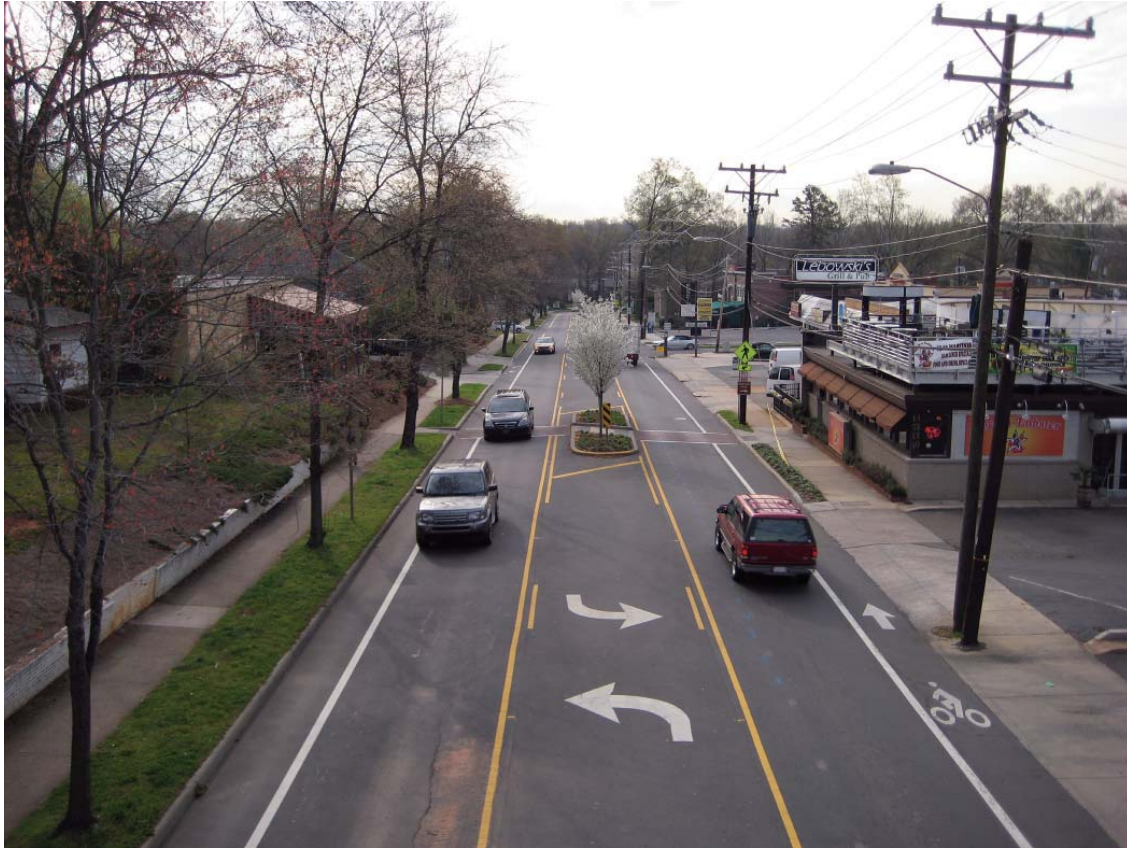
Figure 7-7. Continuous Two-Way Left-Turn Lane
