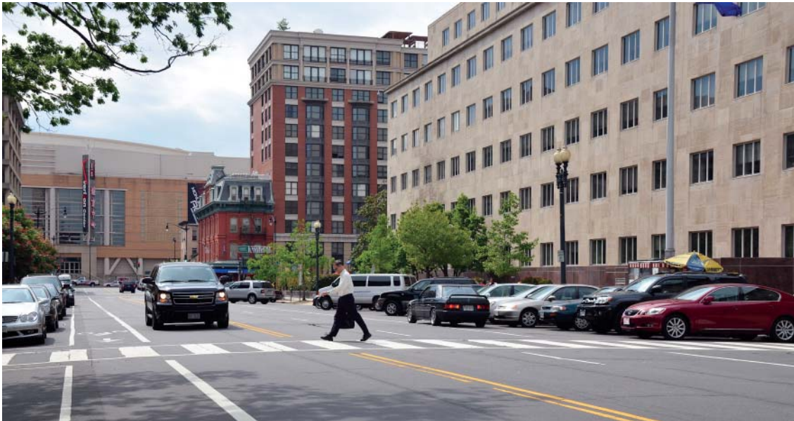
Figure 4-25. Typical Application of Diagonal Back-In/Head-Out Parking
