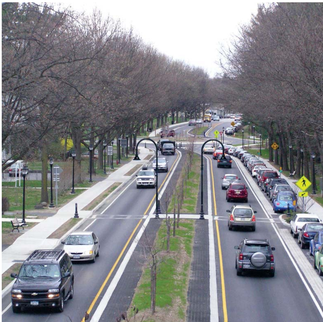
Figure 7-9. Divided Arterial Street with Parking Lane
