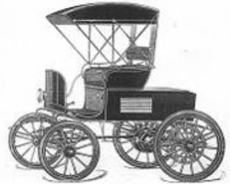
AMERICAN Road Buggy with Top.—Fit two passengers. Front wheels 33 inches, rear wheels 34 inches; speed up to 17 miles per hour.
